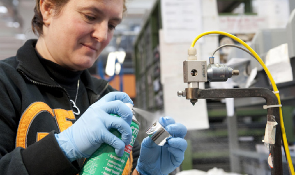
The surface of stainless steel should be carefully prepared before adhesive bonding. Photo: Henkel Loctite, Düsseldorf (D)
