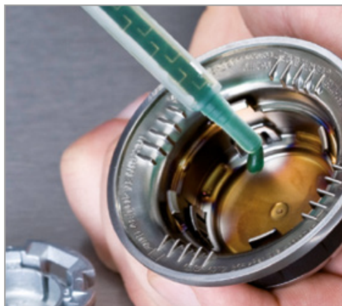
Adhesive bonding provides great flexibility in design.
