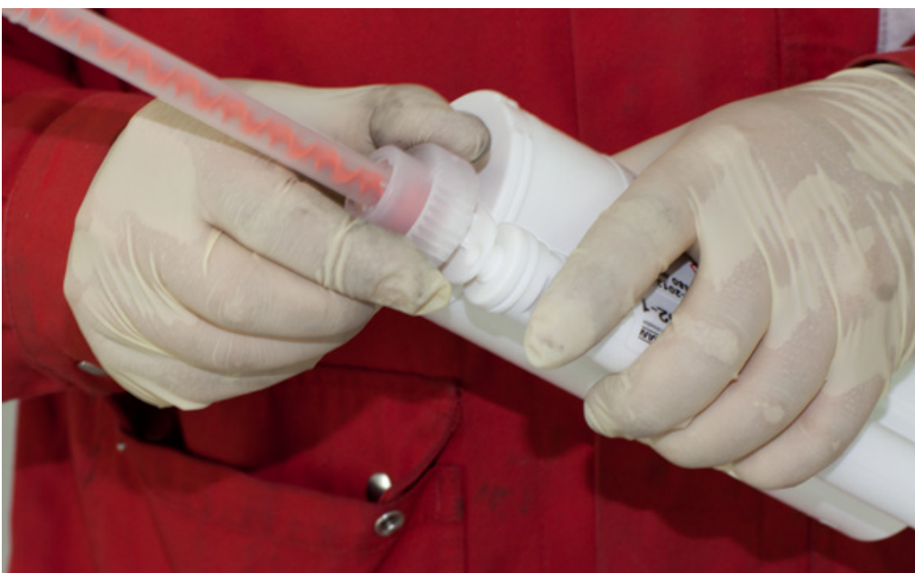
The nozzle is designed in a way that provides the optimal ratio between resin and hardener. Photo: M. Pyper / Arnold, Friedrichsdorf (D)
