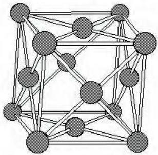
This is called Face Centred Cubic (FCC). There is one atom at each corner and one in the middle of each face. This structure is also called austenitic.
