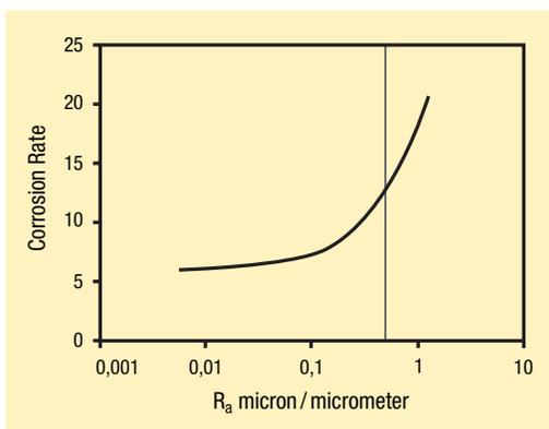
The chart above shows the relationship between corrosion rate and surface roughness. The line represents a surface roughness of  $R_a$  0.5  $\mu\text{m}$  or 20  $\mu\text{in}$ . Corrosion rate accelerated rapidly above this surface roughness level.<sup>3</sup>
