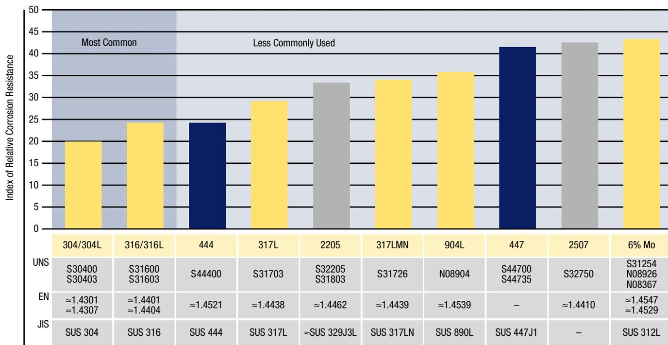
**Figure 1** This chart of relative pitting resistance is based on the Pitting Resistance Equivalent or PRE number. Austenitic stainless steels are shown in yellow, ferritics in blue, and duplex in gray. The UNS (Unified Numbering System), EN (European Number), and JIS (Japanese Industrial Standard) designations identify the specific stainless steel chemistries associated with the common names shown in the bar chart.
